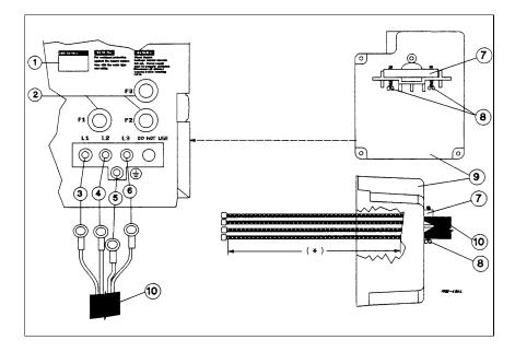
Figure 2-5. Connecting the Series 668xA Power Cord
